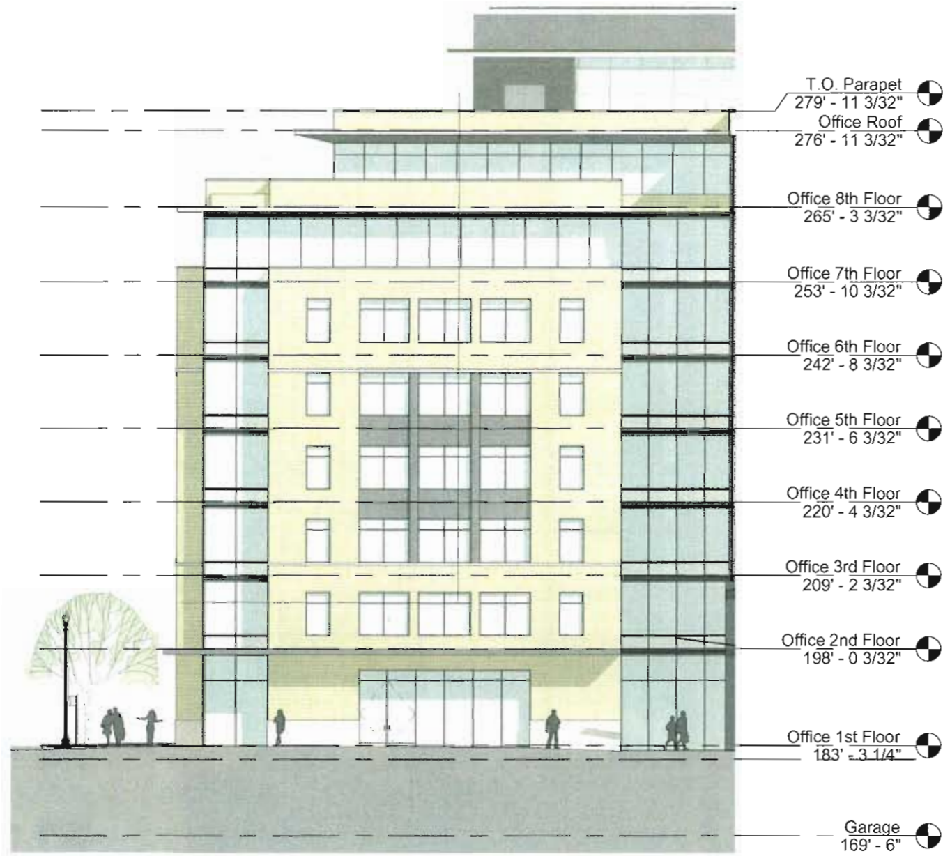
① Front Court East Elevation 1" = 20'-0"
